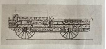
Intended for transporting large numbers of persons across the desert, *Das Wüstenschiff*[*le vaisseau de désert* or, 'desert ship'] was designed as a means to counter the expense and difficulty of constructing roads or railways across vast stretches of uninhabited areas such as the Gobi or the Sahara Desert. Not to be confused with the
